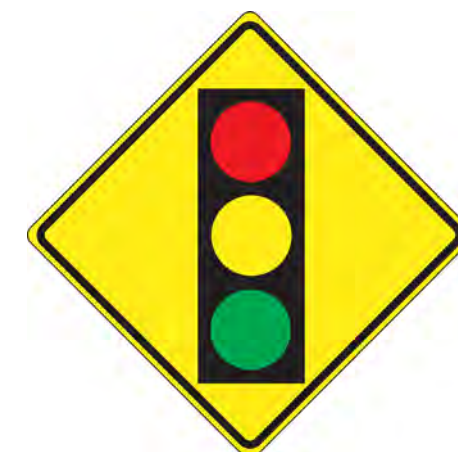
'Signal Ahead Warning' Sign
