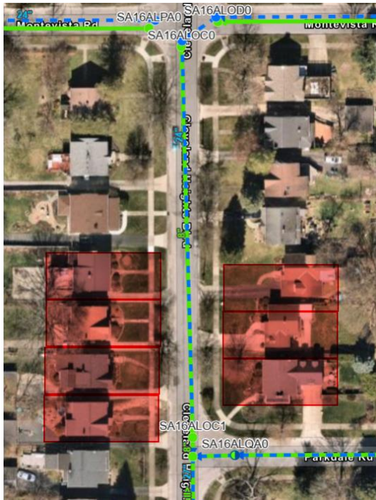
Figure 4: Seven Confirmed Illicit Connections on Cleveland Heights Blvd between Montevista and Parkdale Rd
