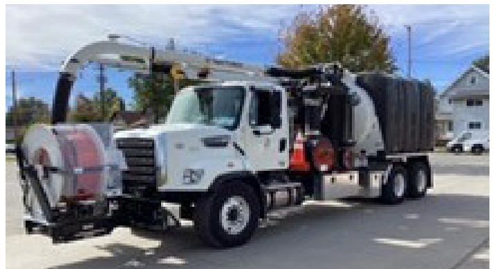
New Sewer Vector Truck
